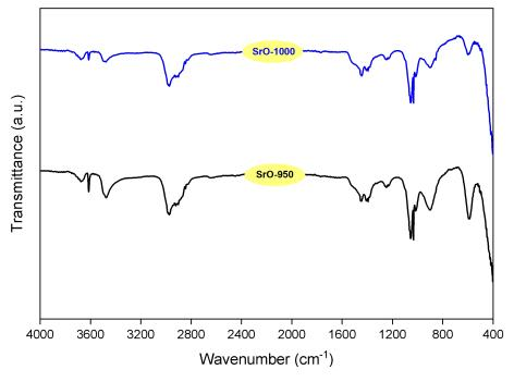
Fig. 2. FTIR results of both SrO samples
