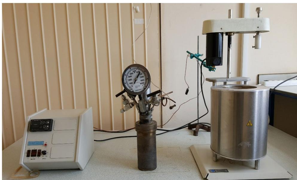
**Figure 1.** The batch reactor used in liquefaction experiments
