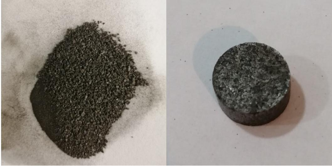
**Fig. 1. a.** Powder form of NiMnCoSn alloy, **b.** Pellet form of NiMnCoSn alloys' powders
