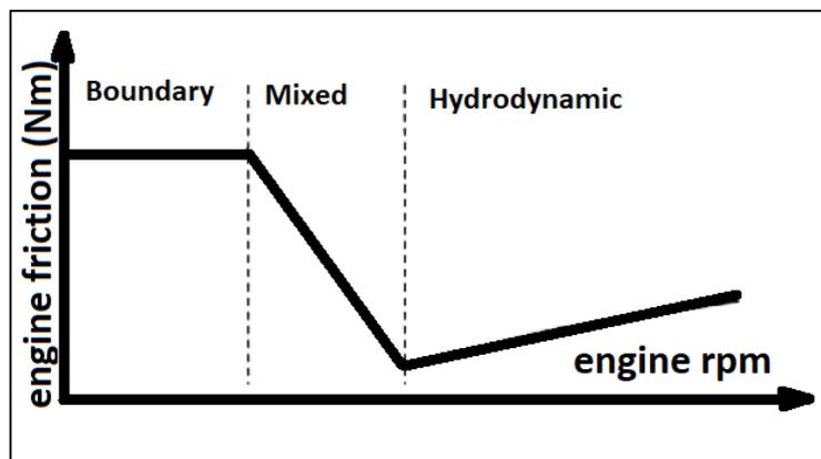
Figure 2. Stribeck Engine Friction Curve
