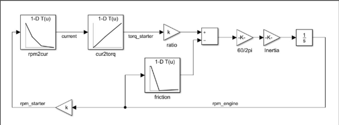
Figure 4. Diesel engine cranking model
