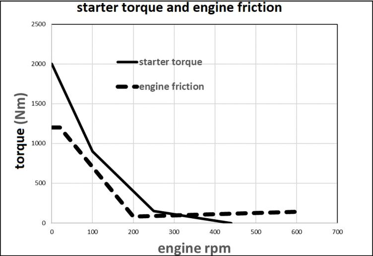
Figure 3. Starter torque and engine friction curves
