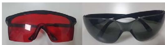
**Figure 1.** While black glasses suitable for Diode laser wavelength should be used, red glasses which previously used for Alexandrite laser were used.
