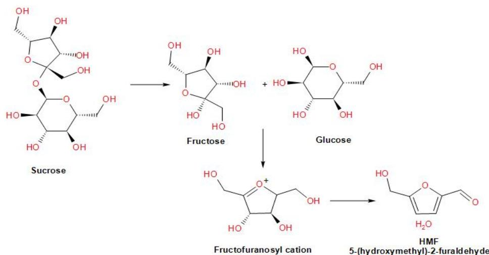
**Fig. 1.** Decomposition of sugars into HMF at elevated temperatures – Maillard Reaction
