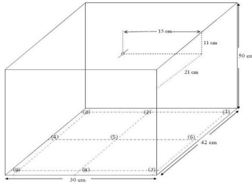
FIGURE 1. Dimensions of the Plexiglas cage used for EMF application and the positions of the nine points used to measure EMF intensity on the Plexiglas cage floor (Keleş et al., 2019).
