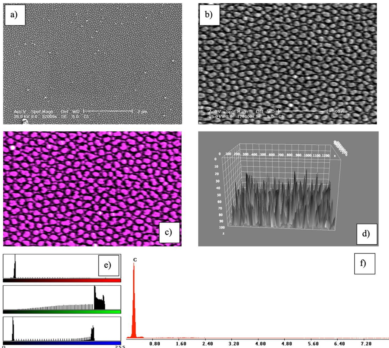
**Figure 2:** (a) SEM images at **32.000x**, (b) SEM images at **128.000x**, (c) SEM image (8-bit/magenta), (d) 3D surface topography, (e) color histogram, and (f) EDS analysis of the carbon nanopillars.
