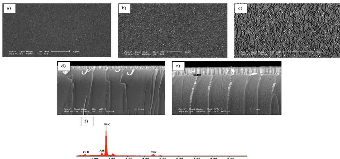
**Figure 1:** (a-b-c) SEM images from the surface (with different magnifications), (d-e) SEM images from the cross-section (with different magnifications), (f) EDS analysis of the prepared AAO template on Si.
